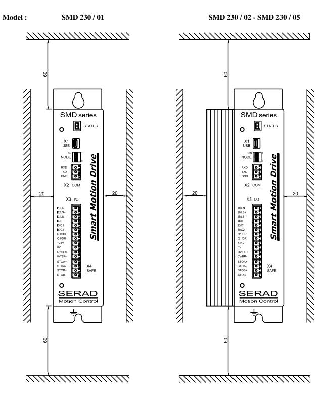
Several drives can be mounted side-by-side provided that enough space (at least 20mm) is left to ensure good natural convection. Leave a space greater than 60mm over and under the drives to allow for the various connectors and cables to be fitted.
