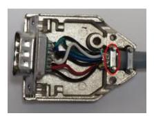
It is highly recommended to use cable with additional shield wire and sold it on the Sub-D:
