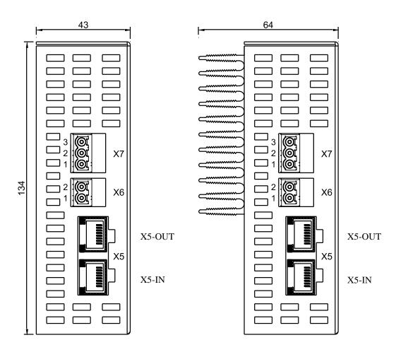
X5 BUS Fieldbus communication (CANopen, EtherCAT)
