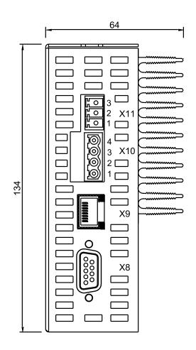
X8 FEEDBACK Main feedback (resolver / Tamagawa encoder / incremental)
